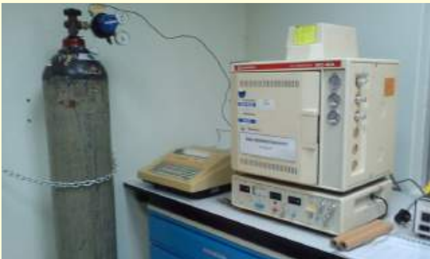
Gas chromatography for hydrogen analysis
