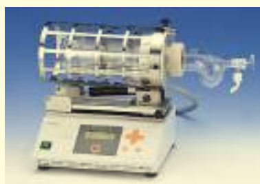
Glass tube oven used for isothermal pyrolysis
