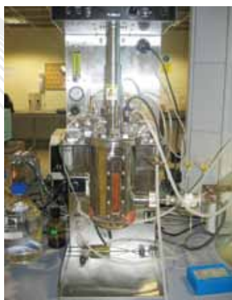
Bioethanol fermentation using hydrolysate of sago hampas in 3L bioreactor
