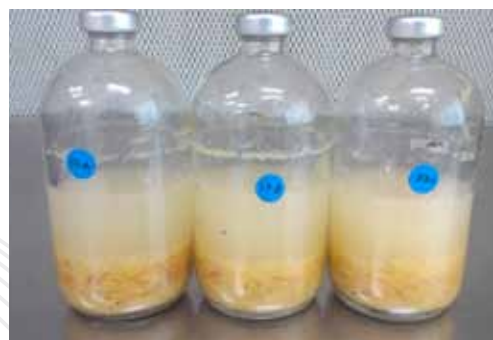
Fermentation of simultaneous saccharification and fermentation for biobutanol production
