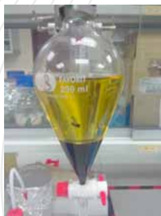
Crude biodiesel product after simultaneous esterification-transfesterification process
