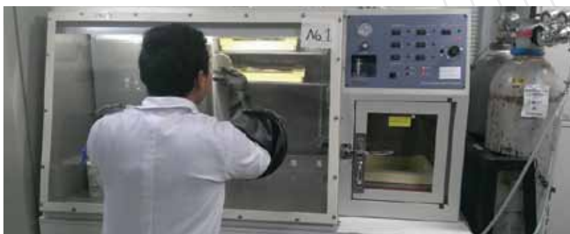
Inoculum was transferred into vials containing media in anaerobic chamber
