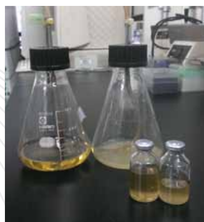
Small serum bottles and anaerobic flask were used for fermentation purpose
