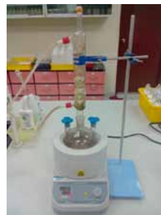
Digital bifunctional heating and stirring mantle used in biodiesel production
