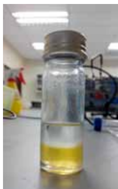
Fatty acids methyl esters, FAME (upper layer) and hexane (lower layer) from used cooking oil
