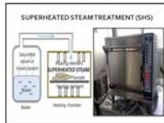
The concept of superheated steam (SHS) treatment.
