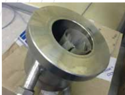
Saturated steam reactor: bottom part
