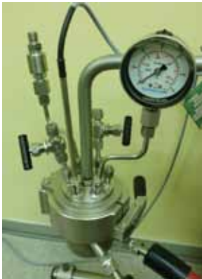
Saturated steam reactor
