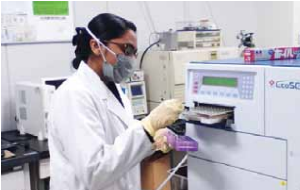
Gel Permeation Chromatography (GPC) analysis of SHS treated PHA samples
