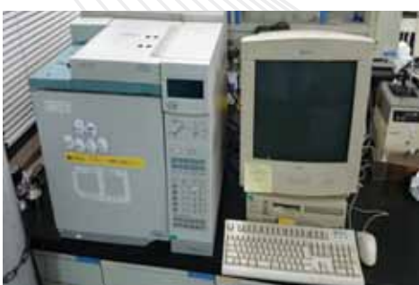
The gas samples were analyzed by gas chromatography
