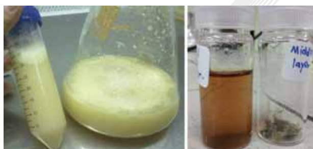
Preparation of dicarboxylic acid monomers from palm oil's fatty acids by fermentation approach
