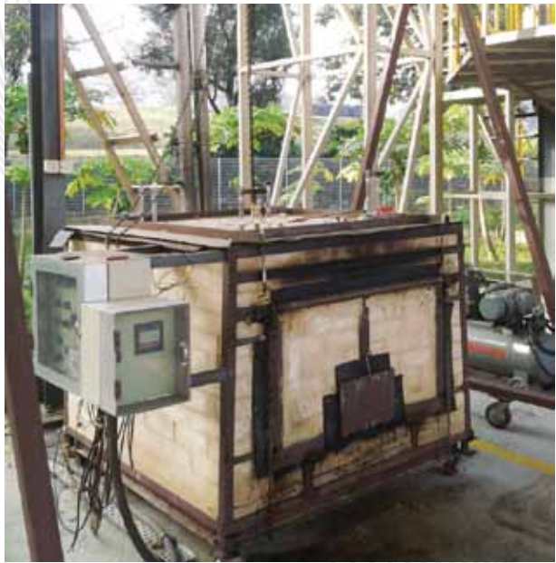
Fig.1 Pilot Scale (30 kg) brick self-sustained carbonization reactor
