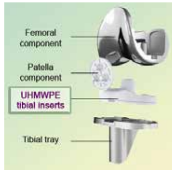
Figure 1: UHMWPE as component of total knee arthroplasty
