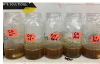
Figure 3. Extraction of phenolic acids from lemongrass leaves using ionic liquid
