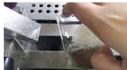
Figure 2: Preparation of PLA/CNF nanocomposite using internal mixer (Brabender)
