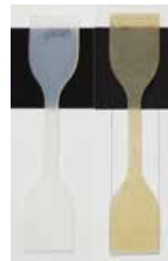
Figure 2: The UHMWPE/CNF nanocomposite and neat UHMWPE
