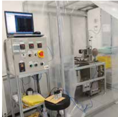
Figure 1 Sand bath reactor system
